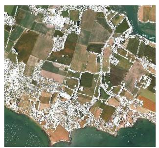
(b) 2.5 m-Vegetation mask (white pixels) superimposed on the orthoimage.
